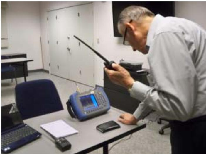
*Gary Hamman, K7GH uses spectrum analyzer to evaluate an HT*
