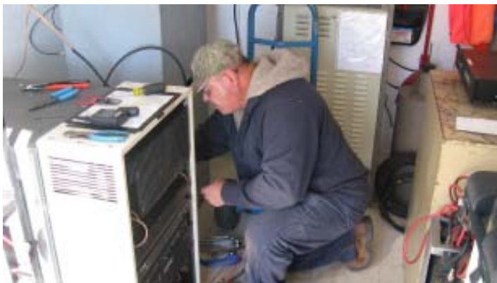
Bill KJ7GYH connecting the Duplexer and Control Antenna cables to the Repeater Cabinet
