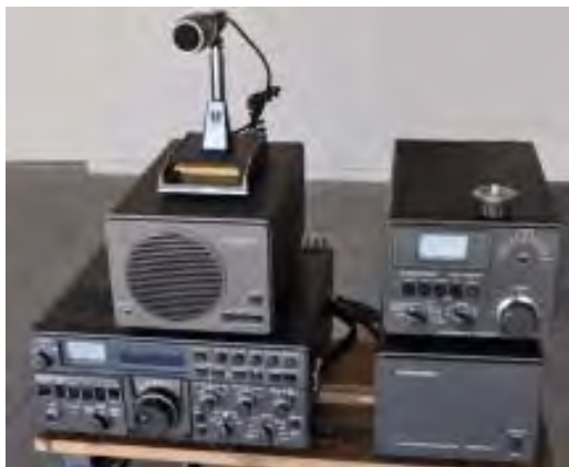
The donated station. A TS-180s radio, speaker, microphone, power supply and antenna tuner.
