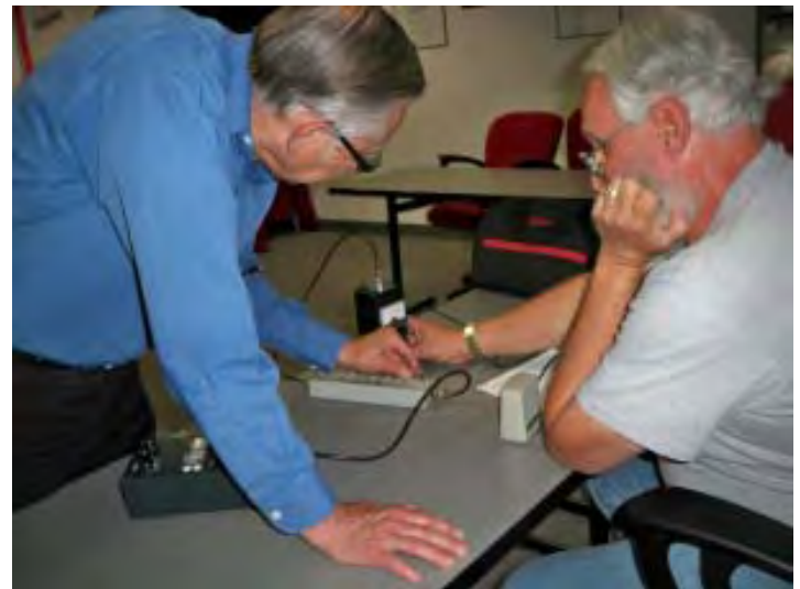
Paul Sharkey, AE7UH, and Gary Hamman, K7GH, test the sensitivity of Paul's home brew field strength meter
